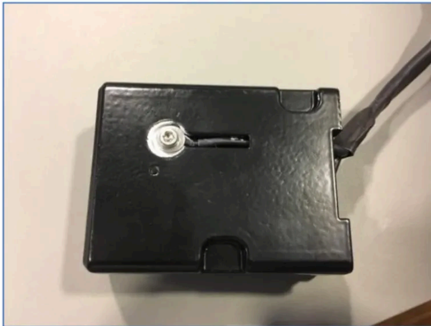
Fig. 18 Sample Heater (PreHeater)
